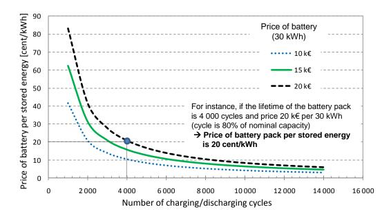
Figure 4—34: Price of battery (30kWh) per charged/discharged energy (snt/kWh) as function of their lifetime (number of charging and recharging cycles)
