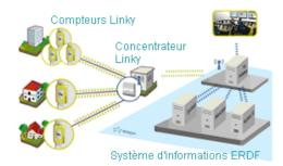
Figure 4—17: ERDF Linky system architecture
