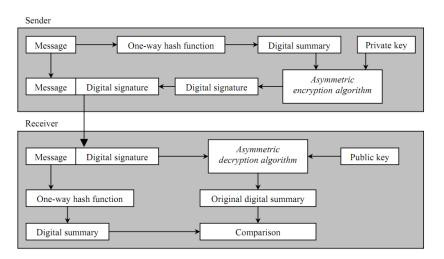
Figure 4–26: The process of creating and verifying digital signature
