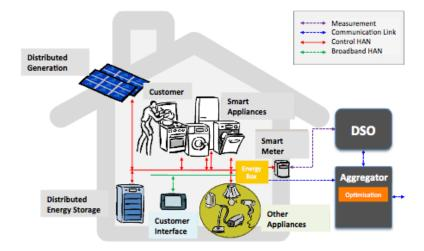
Figure 4—7: General architecture for Active Demand (courtesy of ATLANTIDE, a research project financially supported by *"Ricerca di Sistema"* (Research and Development Projects of general interest for the Electrical System) under the scheme set up by 8<sup>th</sup> March 2006 law)
