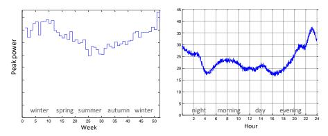
Figure 4—35: Annual (a) and daily (b) load curves of residential customers (electric heating with a water storage)
