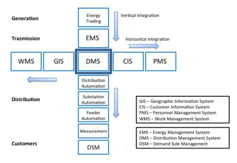
Figure 4—3: Vertical and Horizontal integration of a DMS
