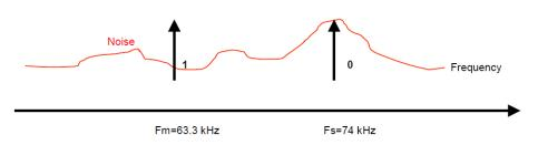
Figure 4—18: Spread-frequency shift keying frequency spectrum
