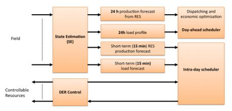
Figure 4—5 – The central DMS architecture proposed in [18]
