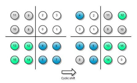
Figure 4—15: DCSK Cyclic Shifting sample performed at symbol 8
