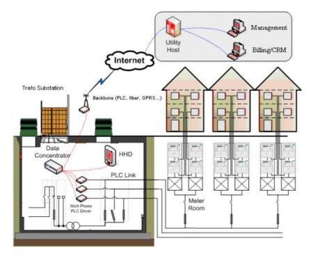
Figure 4—11: PLC Prime reference architecture
