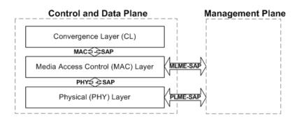
Figure 4—13: PLC PRIME lower layers protocol stack
