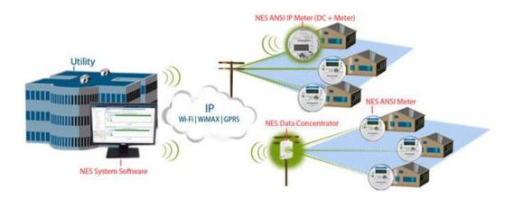
Figure 4—14: Network Energy Service system architecture
