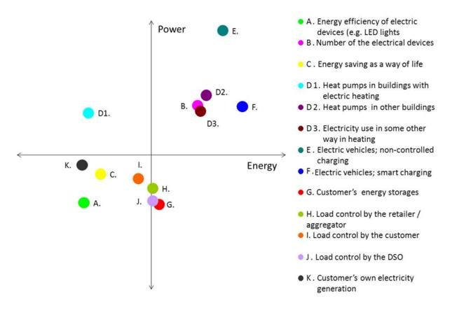
Figure 4—30: Effects of different actions on the power and energy transmitted on the distribution network
