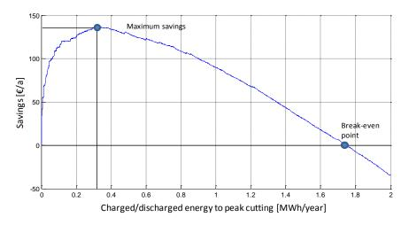
Figure 4—37: Savings vs. needed battery capacity (charging/discharging)
