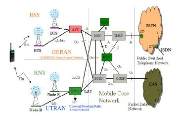
Figure 4–23: Mobile network operator infrastructure
