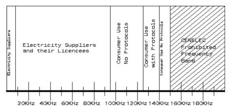
Figure 4—10: Frequency band allocation for PLC networks in Europe
