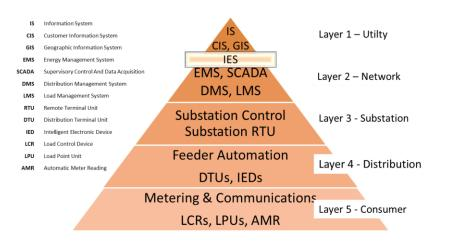
Figure 4–1: The high level architecture of a Smart Grid distribution control centre.
