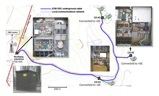
Figure 4—33: Schematic of an LVDC-based electricity distribution system, case Suur-Savon Sähkö, Finland
