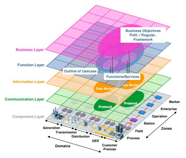
Figure 5—2: Smart Grid Architecture Model (SGAM)
