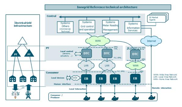
Figure 4—16: InovGrid pilot-project reference architecture
