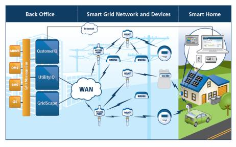
Figure 4–22: RF Mesh Smart Grid architecture
